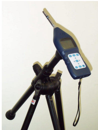
CEL-4627 tripod with CEL-400 sound level meter
